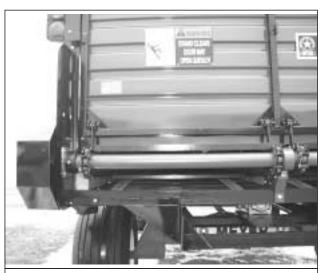
FIGURE 5. DOOR LATCH (Typical both sides)
